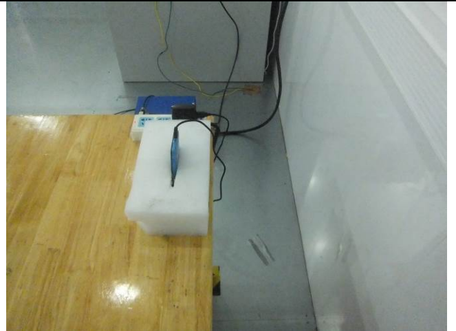
Conducted Emissions Test Setup Side View
