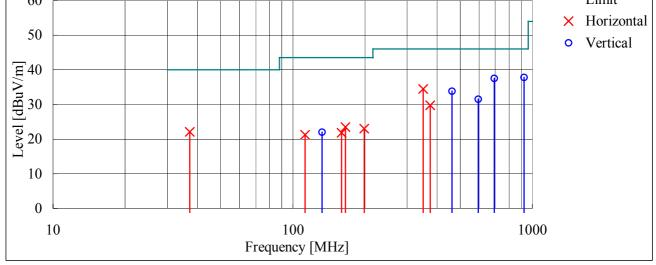
Notes: The test is performed in a distance of 3m. Af : Antenna factor, Cl : Cable loss The test is performed in accordance with ANSI C63.4
