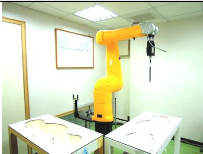
Fig-3.2 SPEAG DASY52 System
