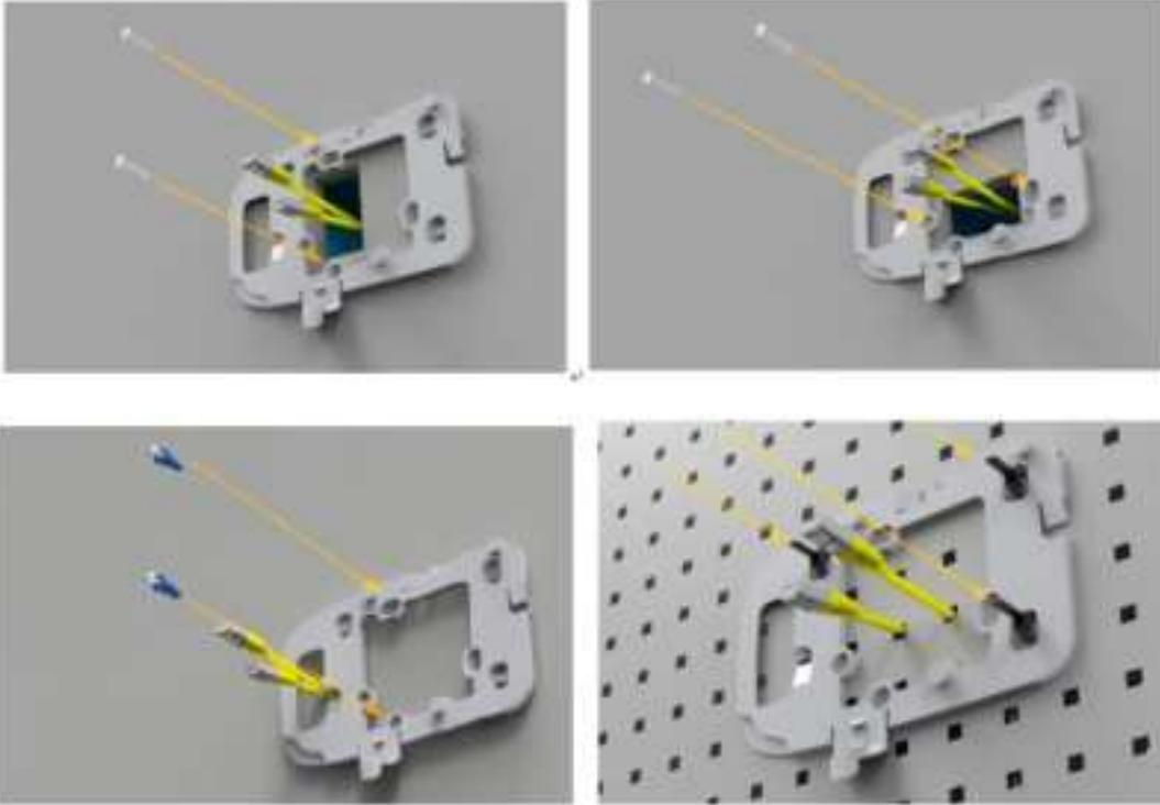
2)Align the wall bracket posts with to the a slot located on the back of the unit .
