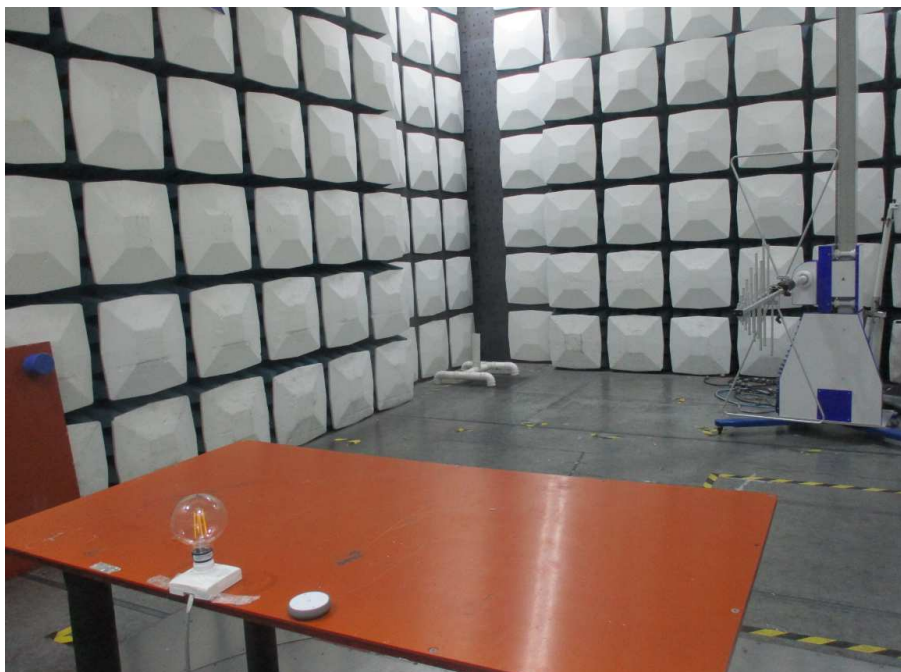
Photograph 2: Set-up for measurement of radiated emission
