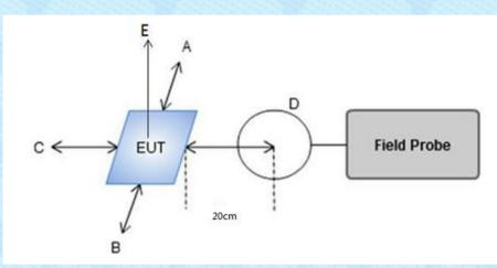
Note: Position A: Front of EUT; Position B: Left of EUT; Position C: back of EUT; Position D: Right of EUT; Position E: Top of EUT(20 cm measure distance)
