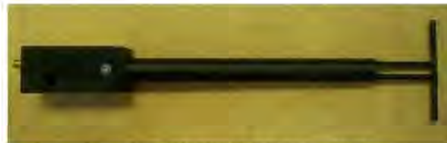
Figure 1 – MVG COMOSAR Validation Dipole
