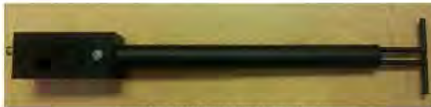
Figure 1 – MVG COMOSAR Validation Dipole
