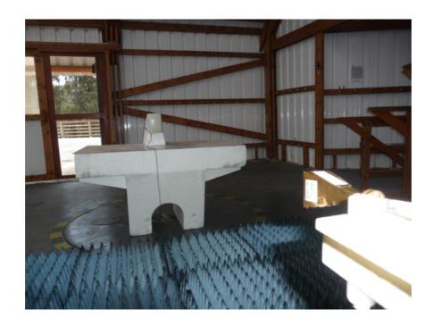
Photograph No.8 Spurious emissions measurement setup at the OATS above 40 GHz
