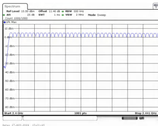
Low End Spectrum Channel Hopping Plot
