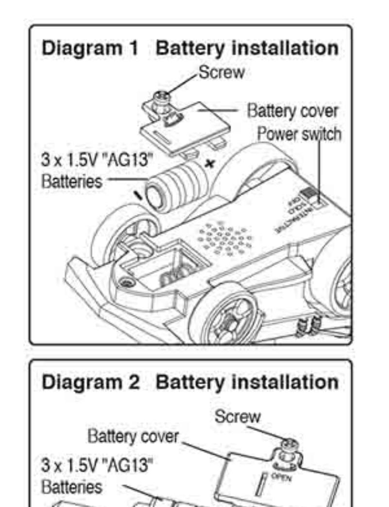
1. Use a screwdriver to loosen the screw on the battery cover and to open the battery cover. (Screwdriver is not included)
