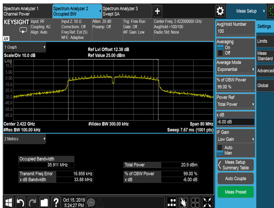
Figure 10 - 2422 MHz 6 dB Bandwidth and 99 % Occupied Bandwidth
