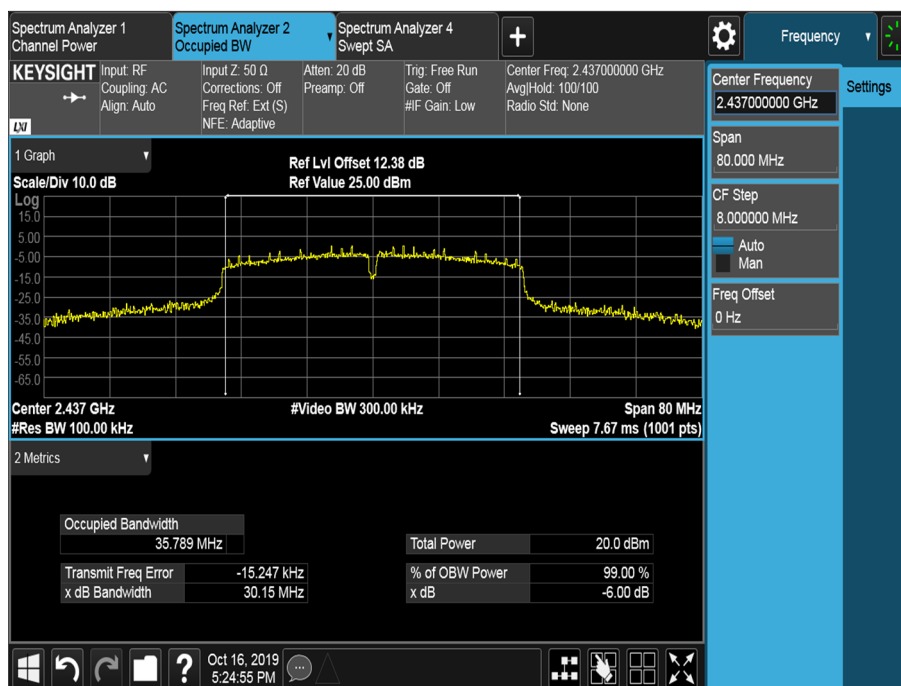
Figure 11 - 2437 MHz 6 dB Bandwidth and 99 % Occupied Bandwidth
