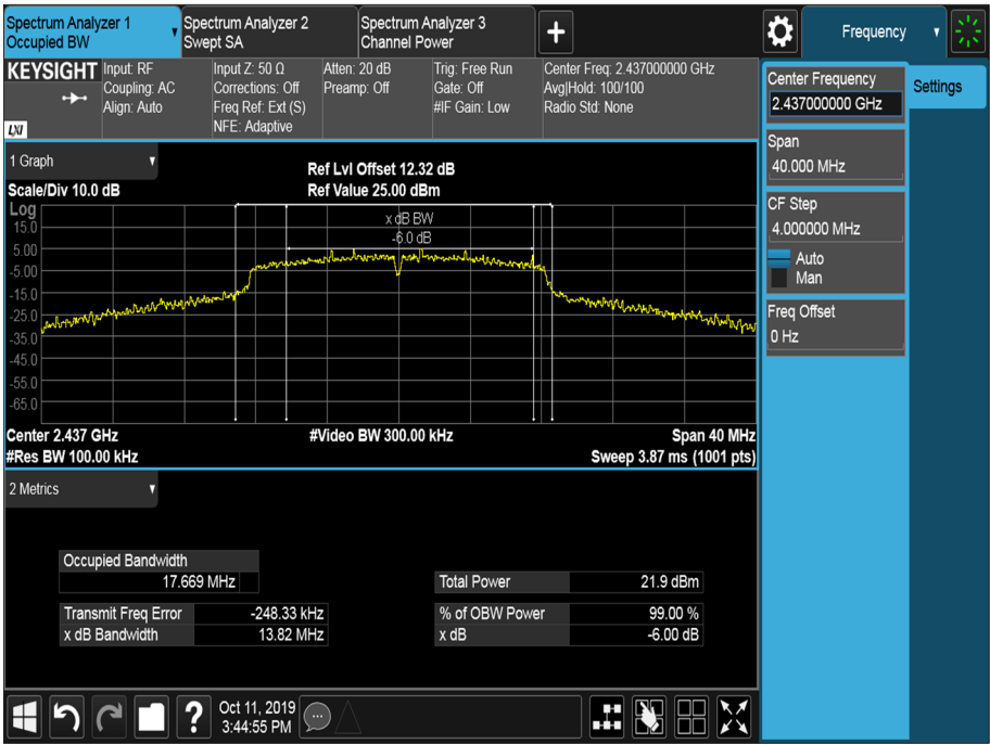
Figure 5 - 2437 MHz – 6 dB Bandwidth and 99 % Occupied Bandwidth
