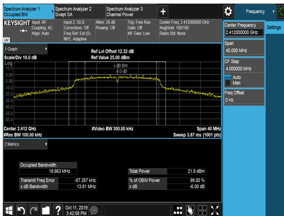
Figure 4 - 2412 MHz – 6 dB Bandwidth and 99 % Occupied Bandwidth
