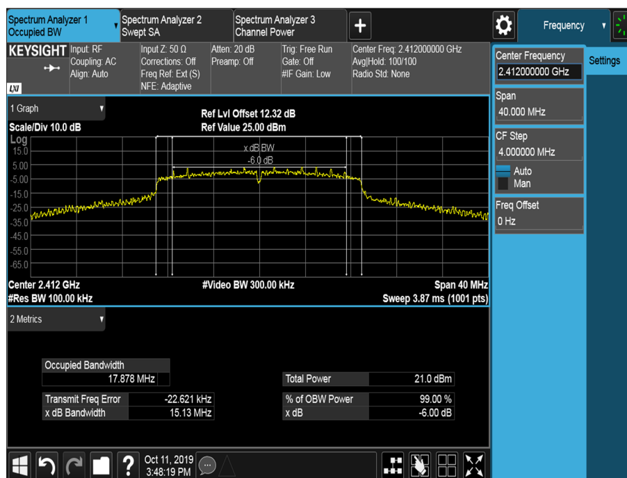
Figure 7 - 2412 MHz 6 dB Bandwidth and 99 % Occupied Bandwidth
