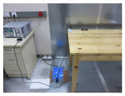
FCC RADIATED EMISSION TEST SETUP
