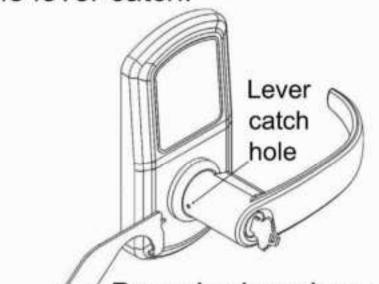
Removing inner lever insert tool into lever catchholt & push back the lever catch, remove lever.
