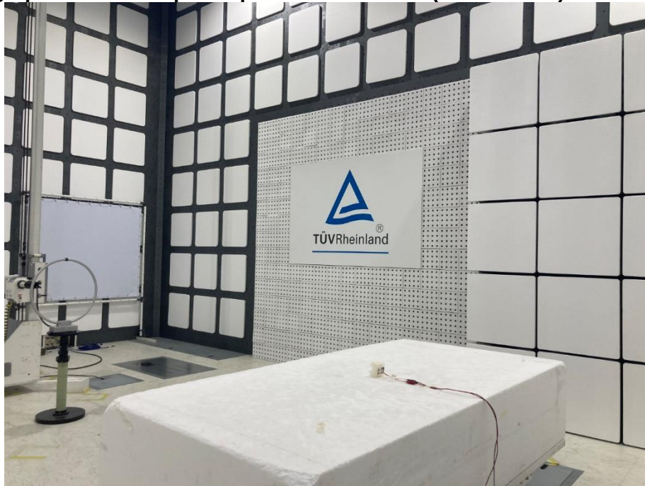
Photograph 4: Test Setup for Spurious Emissions (Back View 2)
