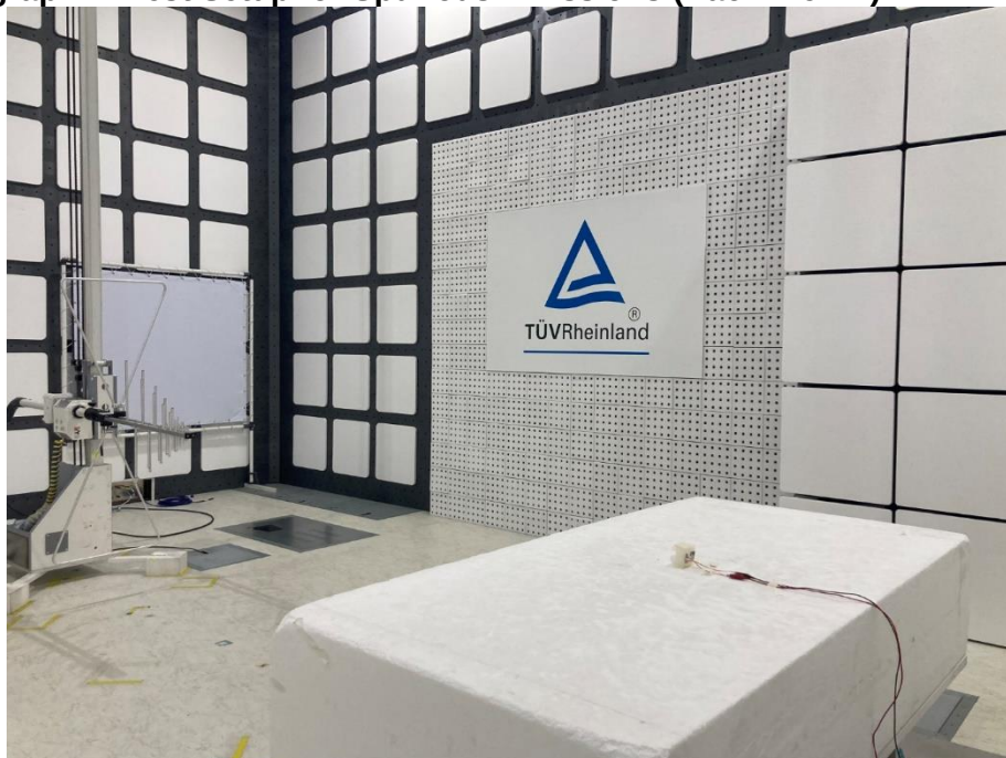
Photograph 4: Test Setup for Spurious Emissions (Back View 2)
