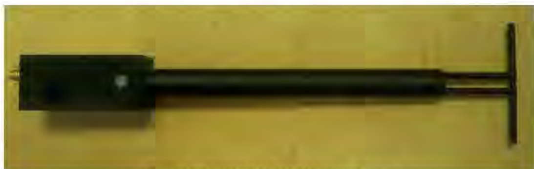
Figure 1 – MVG COMOSAR Validation Dipole
