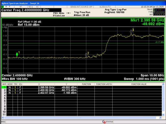
Out Of Band Emission(Left) \pi/4 DQPSK_2-DH5_Channel Hopping
