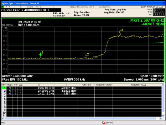
Out Of Band Emission(Left) 8DPSK_3-DH5_Channel Hopping
