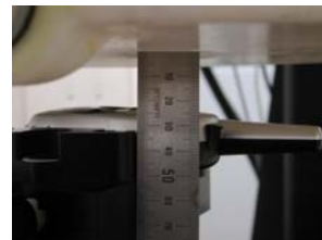
Figure 11. Mouth Face SAR Test Setup
