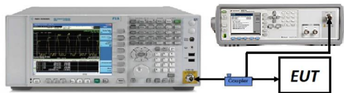
Figure 7-6. Test Instrument & Measurement Setup
