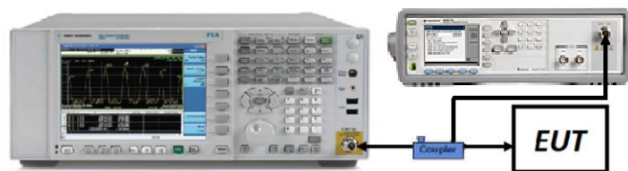
Figure 7-7. Test Instrument & Measurement Setup
