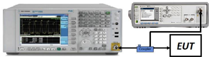
Figure 7-4. Test Instrument & Measurement Setup
