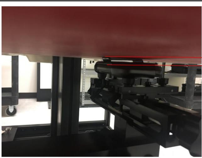
SAR set up View (with case: Distance>15mm)
