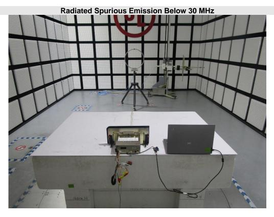
Radiated Spurious Emission Below 1 GHz and 30 MHz
