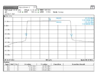
40 MHz 3 Modulation: 256QAM
