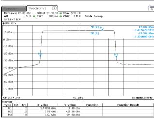
40 MHz 1 Modulation: 256QAM
