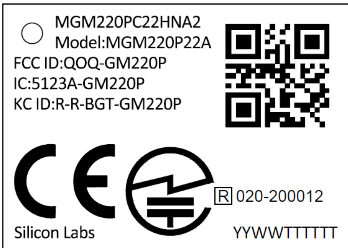
Figure 1: Label / Top Markings of MGM220P22A
