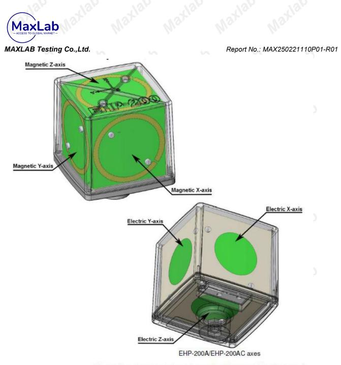
The sensitive elements are located approximately 8 mm below the external surface
