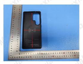
Transmitter to top: $2\pm0.5$ mm Transmitter to Bottom: $11\pm0.5$ mm Transmitter to Left: $37\pm0.5$ mm Transmitter to Right: $37\pm0.5$ mm Transmitter to Front: $85\pm0.5$ mm Transmitter to Rear: $75\pm0.5$ mm
