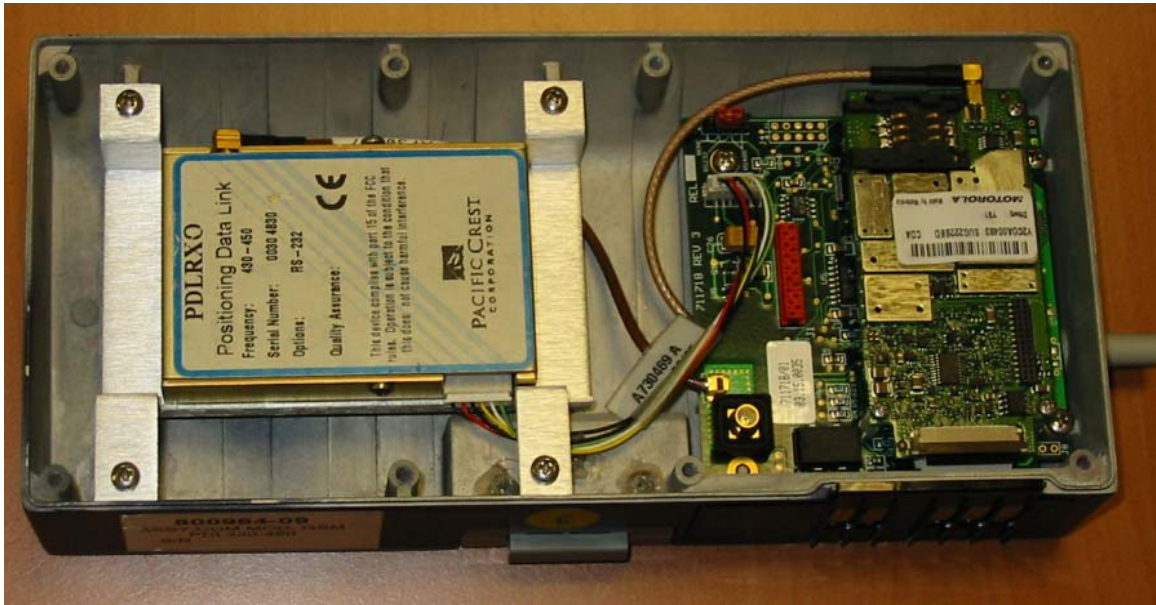
GSM module and Pacific Crest Receiver installed in the Com Module
