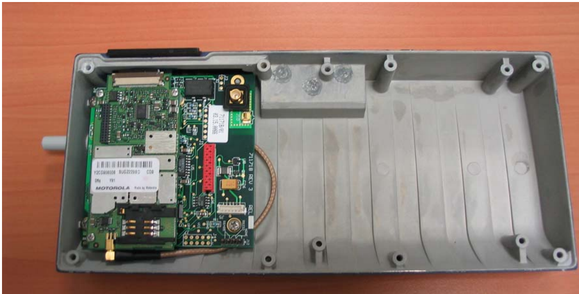
Internal view of Com Module showing location of GSM module mounted to control circuit board (note, no receiver module installed in top photograph).
