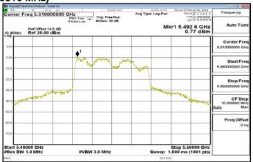
Maximum Power Spectral Density Data Plot (CH Mid 5550 MHz)
