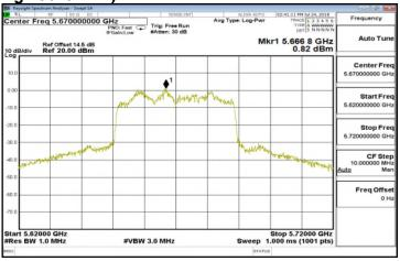
Maximum Power Spectral Density Data Plot (CH **High 5710 MHz)**
