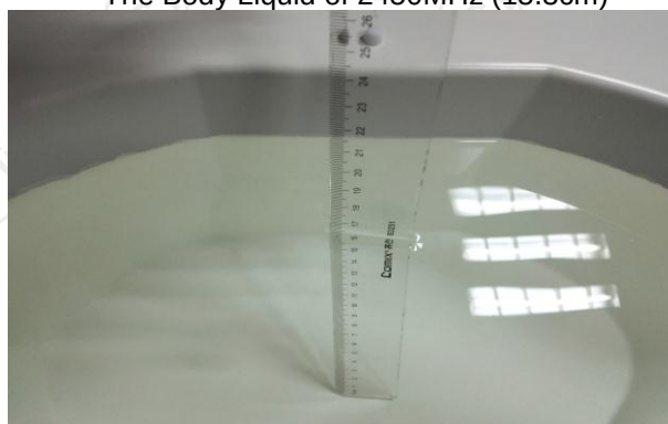
The Body Liquid of 5000-6000MHz (16.5cm)
