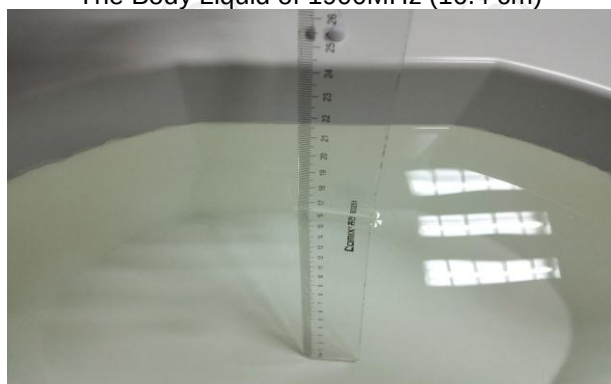
The Body Liquid of 2600MHz (16.5cm)
