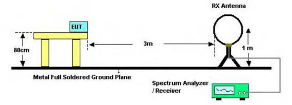
(B) Radiated Emission Test Set-Up Frequency Below 1 GHz
