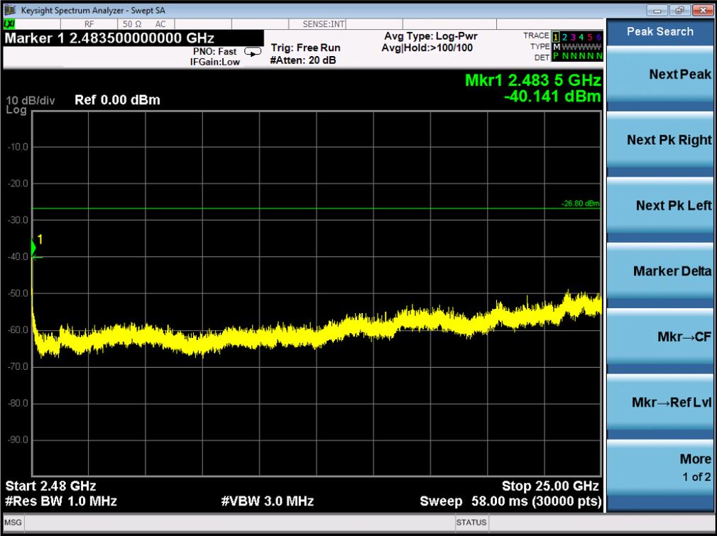
Note: The 100kHz RBW used in the conducted spurious test from 2.4835GHz to 25GHz may result in long measuring times, To avoid such long measuring times, the 1MHz RBW can be used for pre-test. If the emission level exceeded the limit at one or more frequencies, the 100kHz RBW would be used for final test at the special frequency.
