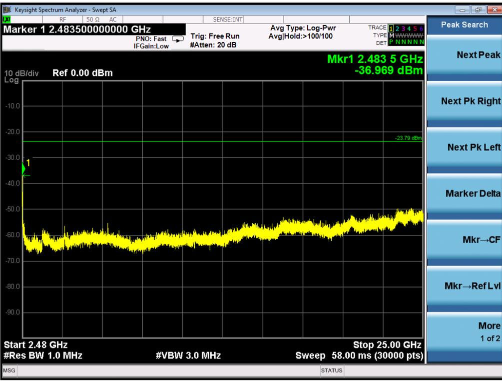
TEST PLOT OF OUT OF BAND EMISSIONS THE WORST CASE
