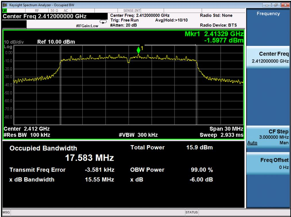
**TEST PLOT OF BANDWIDTH FOR MIDDLE CHANNEL**
