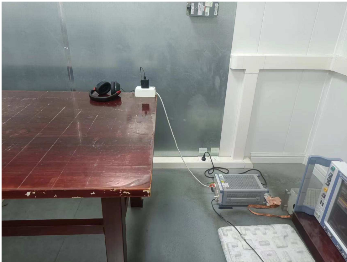
Photograph 3: Set-up photo for Conducted Emission
