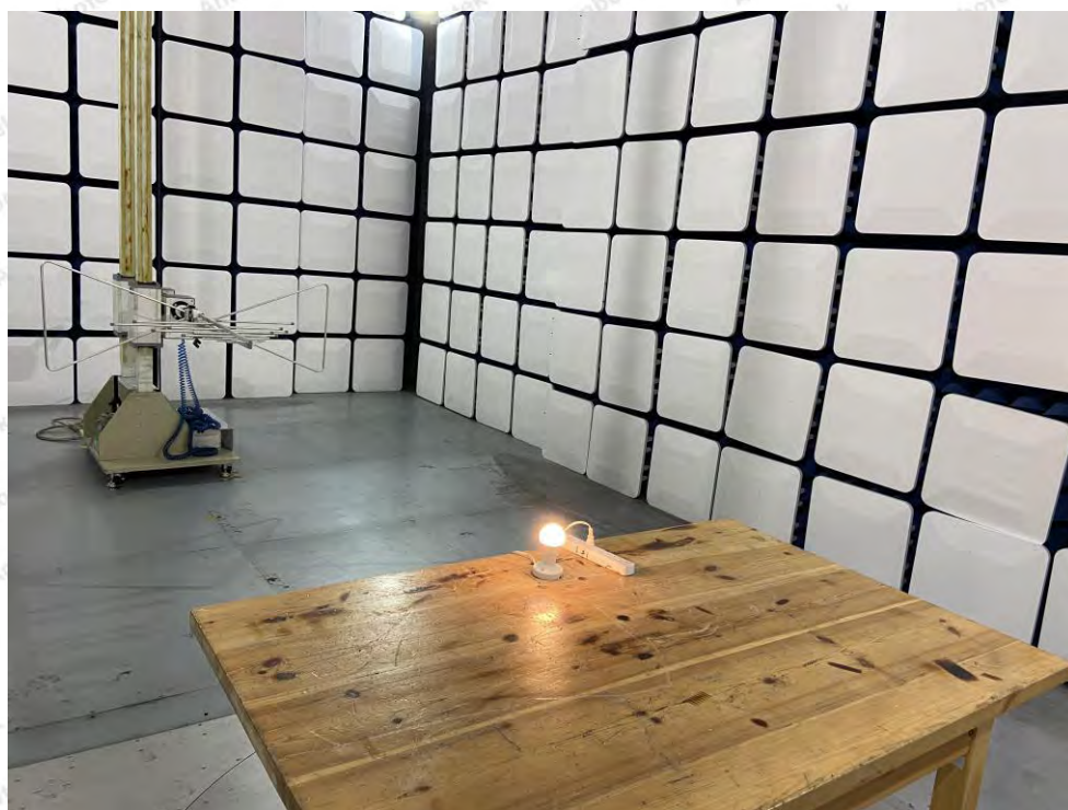
Photo of Radiation Emission Test
