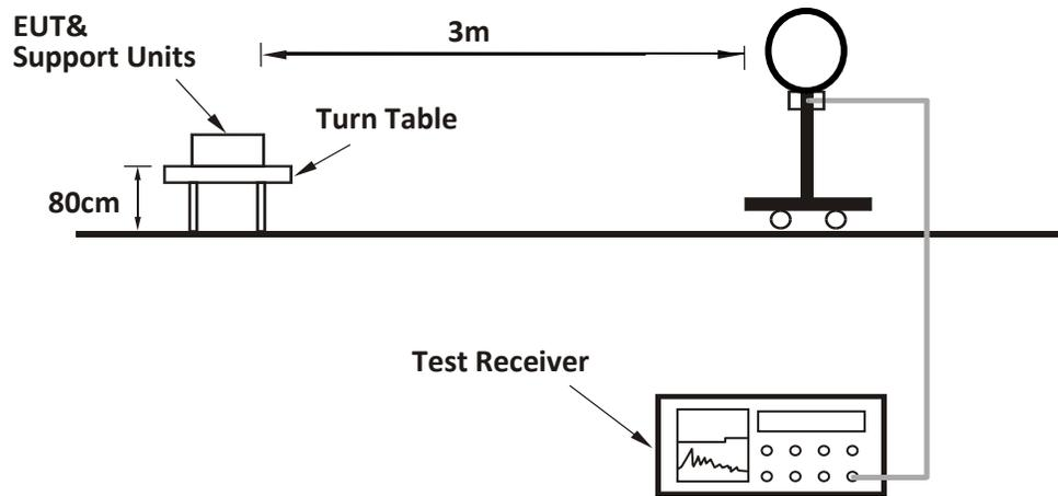
For Radiated emission 30MHz to 1GHz:
