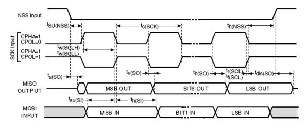
\* 1. Measurement points are done at CMOS levels: 0.3 VDDand 0.7 VDD.
