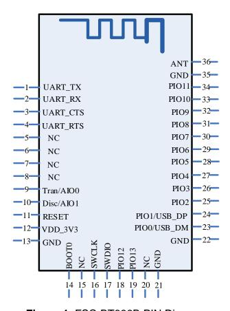
Figure 1: FSC-BT836B PIN Diagram
