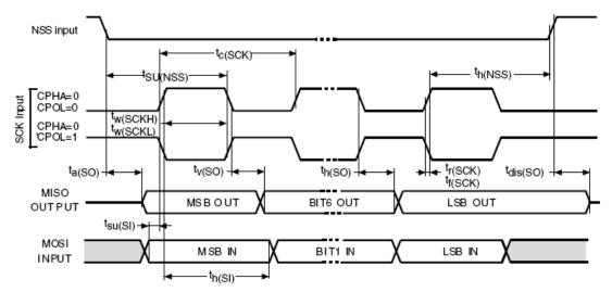
Figure 3: SPI timing diagram - slave mode and CPHA = 0
