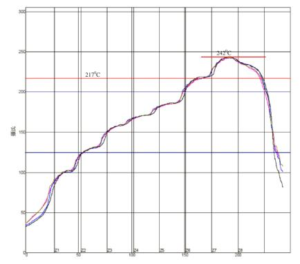
Figure 9: Typical Lead-free Re-flow
