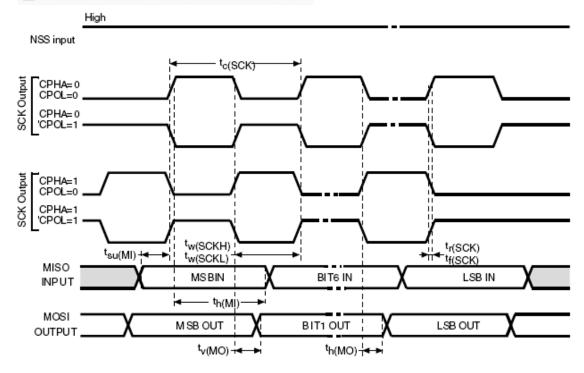
1.Measurement points are done at CMOS levels: 0.3 VDD and 0.7 VDD
