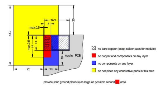
Figure 6: FSC-BT836B Restricted Area
