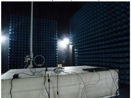
Radiated Emission Set up Photos (Below 1GHz)
