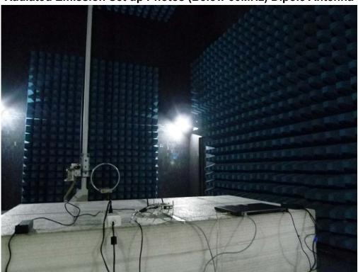
Radiated Emission Set up Photos (Below 1GHz)
