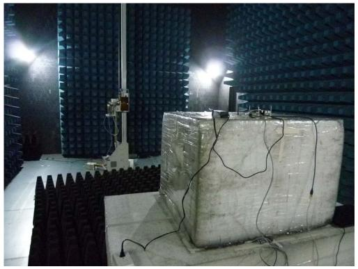
Radiated Emission Set up Photos (Front View)
