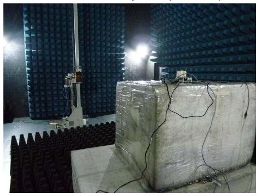
Radiated Emission Set up Photos (Front View)
