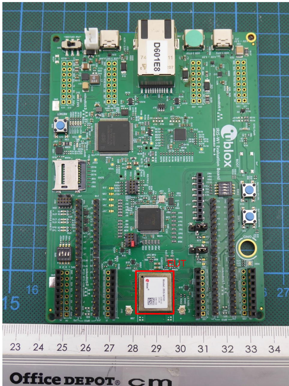
IRIS-W101-00B on evaluation board – top view
