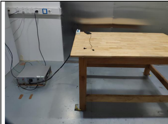
Conducted Emissions Test Setup Front View
