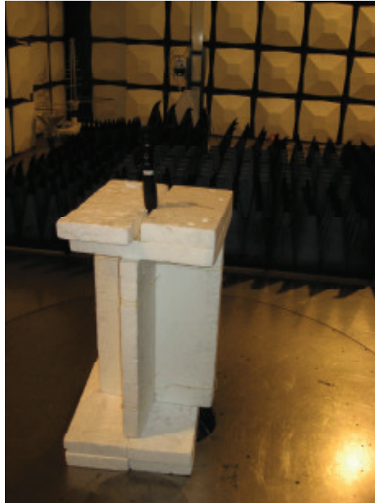
Photograph 2: Set-up for Radiation Measurement above 1GHz
