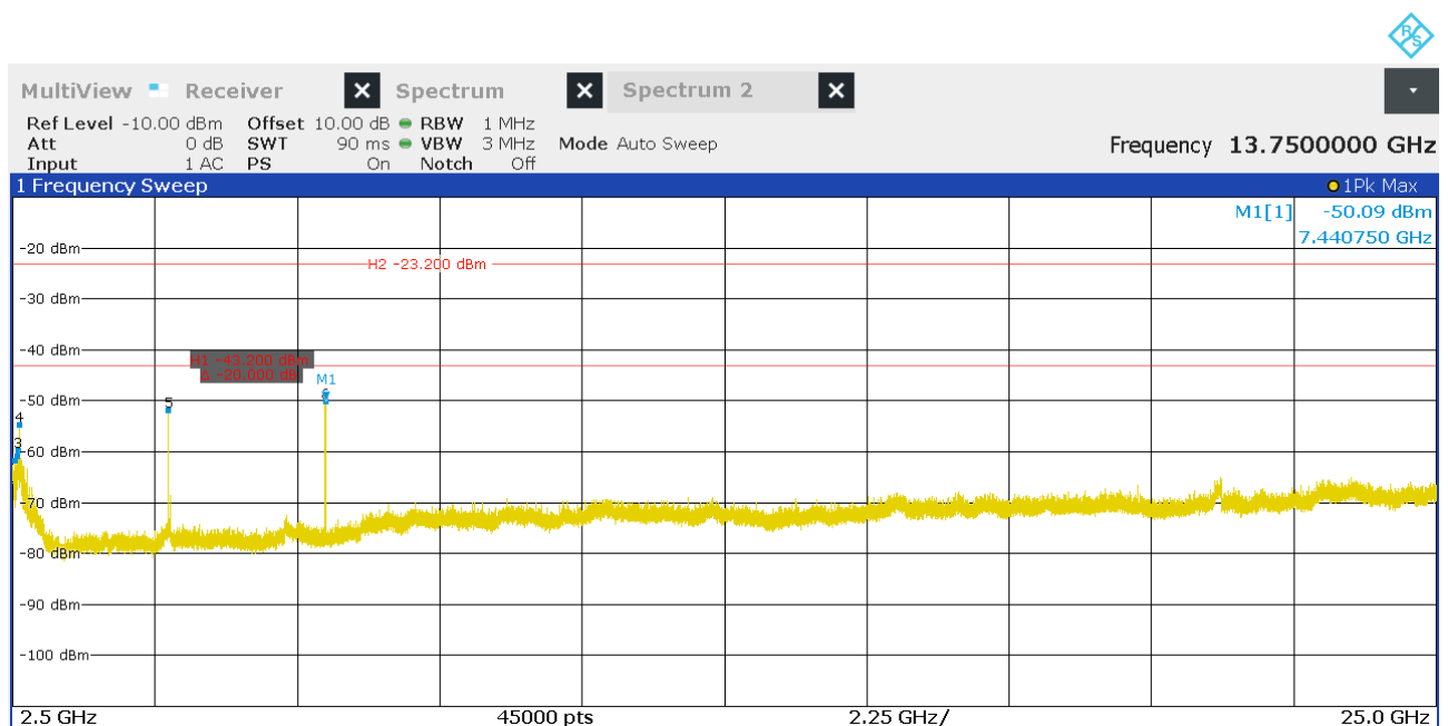
Figure 32: Chart of emissions test from 2.5 GHz to 25 GHz on highest channel, Pk
