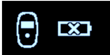
Figure 67: Low Charger Battery Alert Screen
