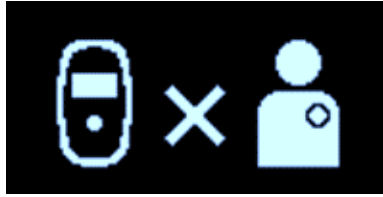
Figure 56: Charger/IPG Pairing Error Screen
