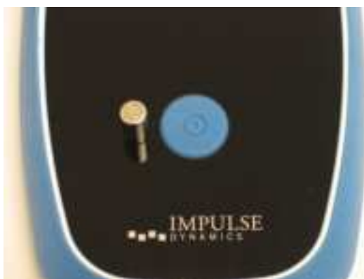
Figure 76: Pairing Magnet on Vesta Charger
