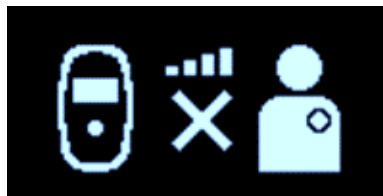
Figure 61: Charging IPG Coupling Error Screen
