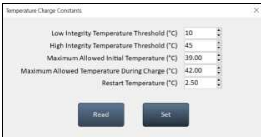
Figure 47: Temperature Charge Constants Window
