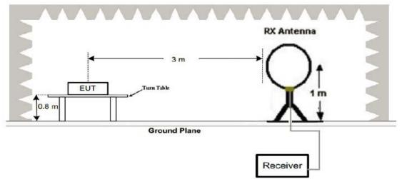
(2) Radiated Emission Test-Up Frequency 30MHz~1GHz
