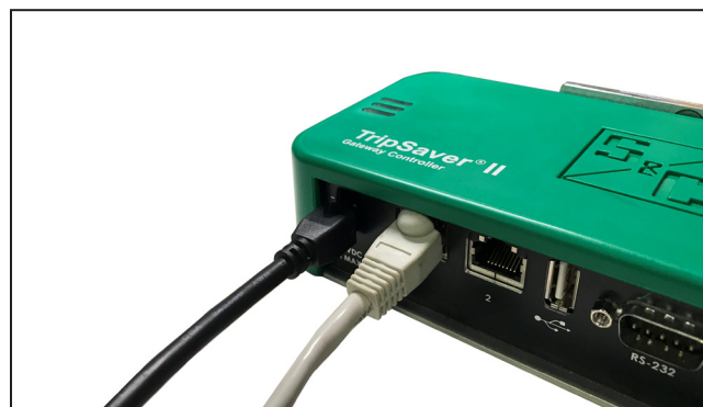
Figure 4. Connecting the gateway controller to ac power and Ethernet 1 port.
