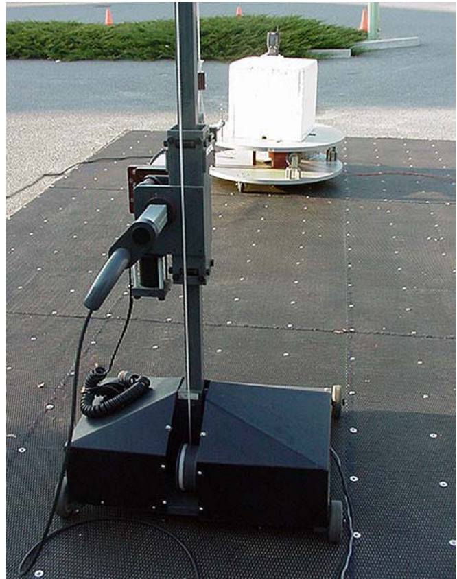
Cellular Band - Dipole Receive Antenna - Vertical Polarization
