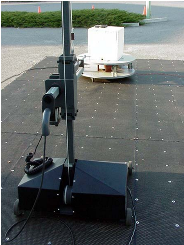
Cellular Band - Dipole Receive Antenna - Horizontal Polarization
