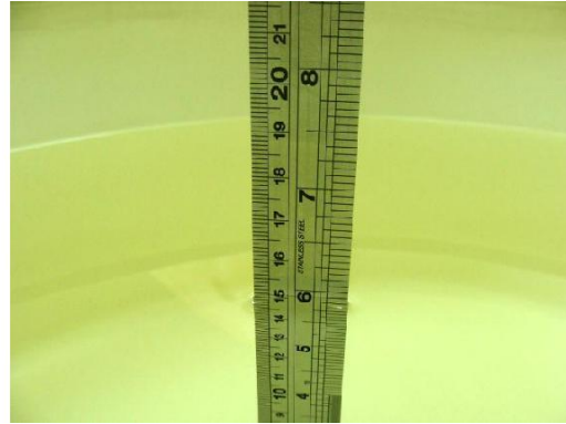
Fig 7.2 Photo of Liquid Height for Body SAR
