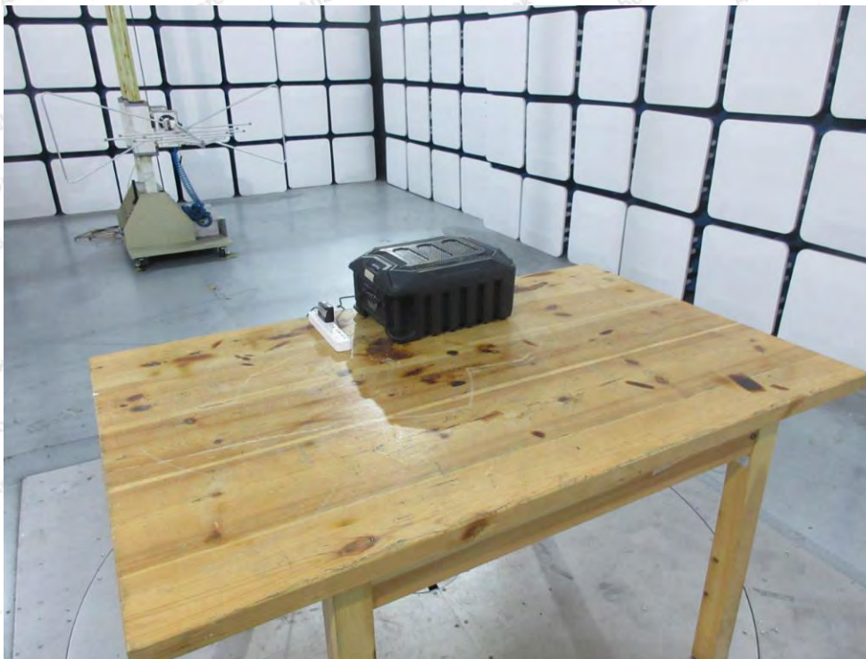
Photo of Radiation Emission Test
