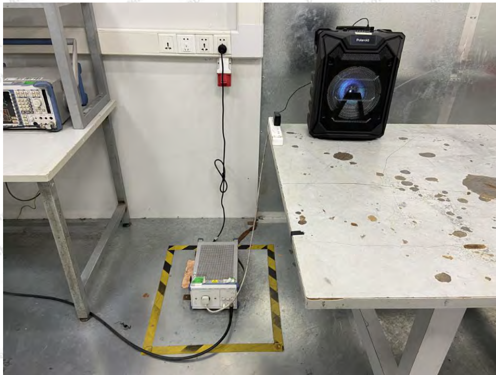
Photo of Power Line Conducted Emission Test
