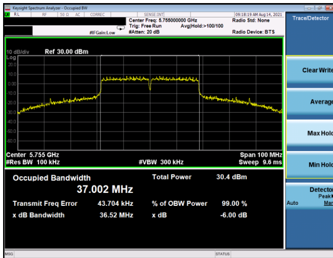
Plot 7-195. 6dB BW & 99% OBW Antenna 3b (40MHz BW 802.11n - Ch. 151, MCS5)
