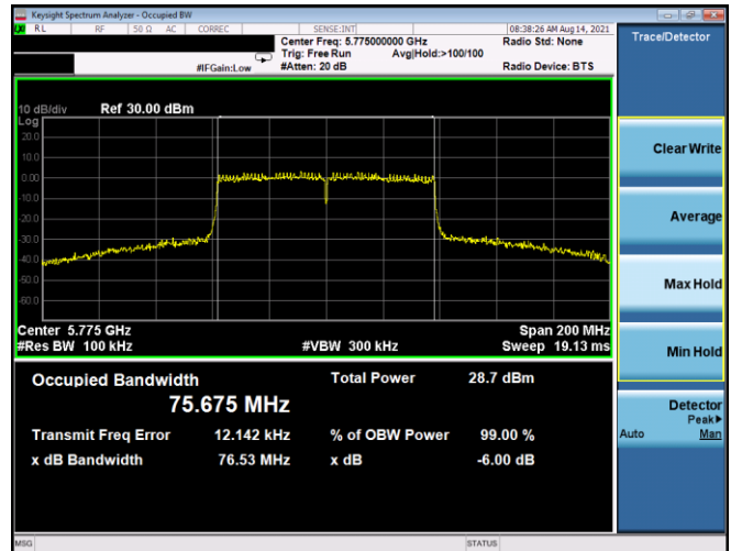
Plot 7-179. 6dB BW & 99% OBW Antenna 5T (80MHz BW 802.11ac – Ch. 155, MCS5)
