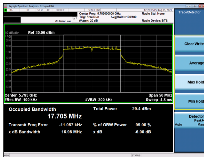
Plot 7-199. 6dB BW & 99% OBW Antenna 1b (20MHz BW 802.11n - Ch. 157, MCS2)
