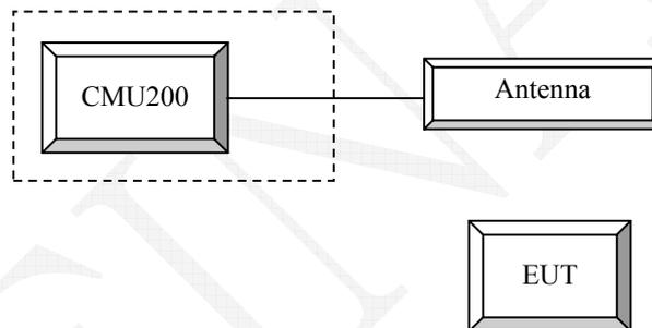
**Block Diagram of Test Setup**
