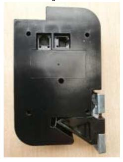
The lock has 2 RJ12 connectors, both are identical:
