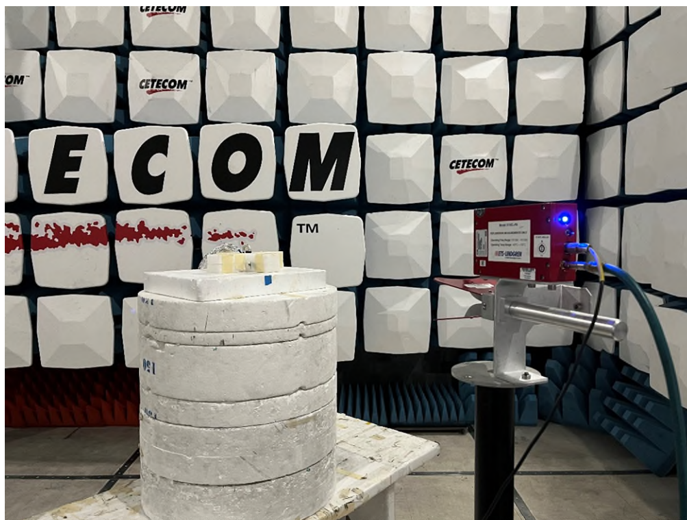
Photo 5: Emissions in frequency range 18-40 GHz
