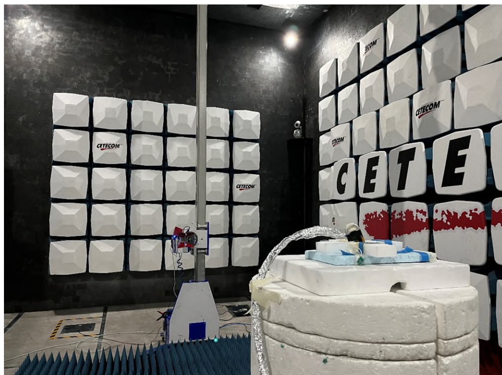
Photo 4: Emissions in frequency range 3-18 GHz
