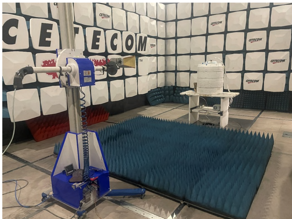
Photo 3: Emissions in frequency range 1-3 GHz
