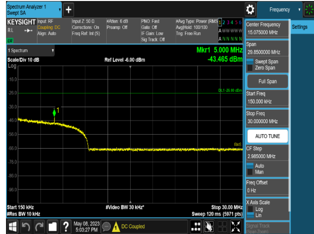
Plot 8-586. Conducted Spurious Emission Plot 150 kHz to 30 MHz
