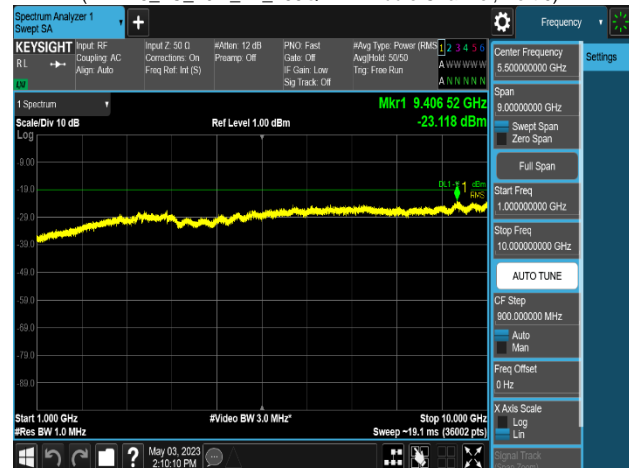
Plot 8-627. Conducted Spurious Emission Plot 1 GHz to 10 GHz (LTE B5_1C_10M_4T_256QAM - Middle Channel, Port 0)
