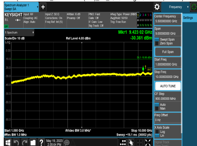
Plot 8-596. Conducted Spurious Emission Plot 1 GHz to 10 GHz
