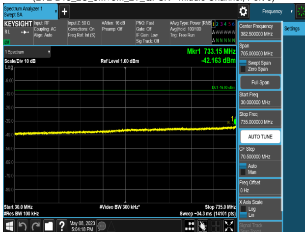
Plot 8-587. Conducted Spurious Emission Plot 30 MHz to 735 MHz
