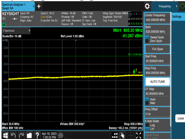
Plot 8-636. Conducted Spurious Emission Plot 30 MHz to 858 MHz
