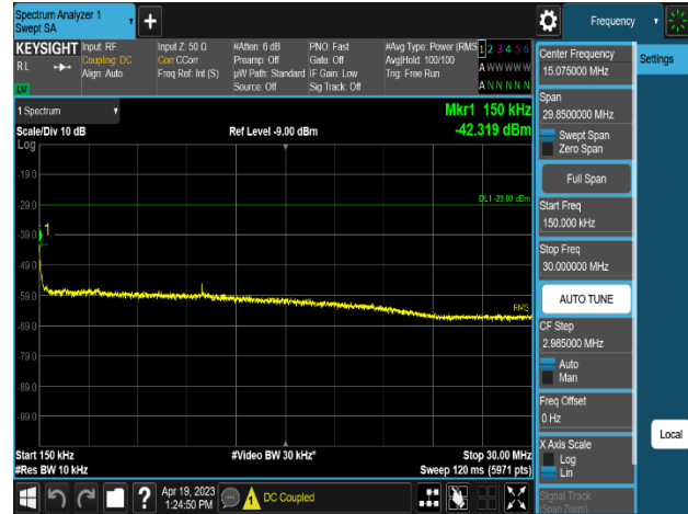
Plot 8-635. Conducted Spurious Emission Plot 150 kHz to 30 MHz
