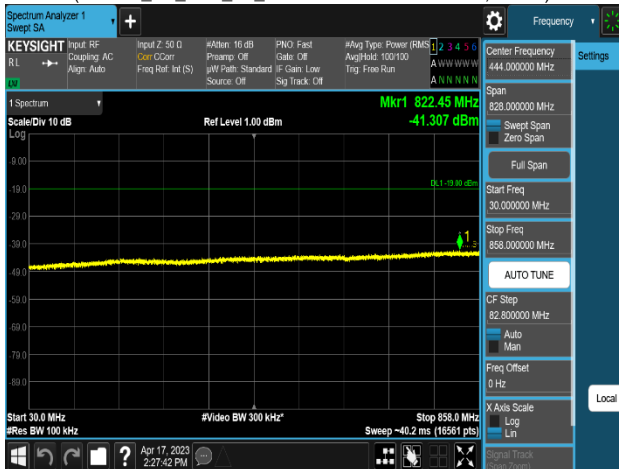
Plot 8-624. Conducted Spurious Emission Plot 30 MHz to 858 MHz (LTE B5_1C_10M_4T_256QAM - Middle Channel, Port 0)
