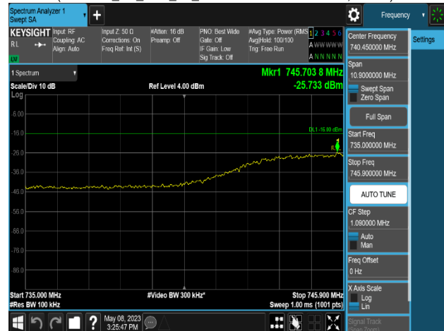
Plot 8-582. Conducted Spurious Emission Plot 735 MHz to 745.9 MHz (LTE B13_1C_10M_2T_64QAM - Middle Channel, Port 0)
