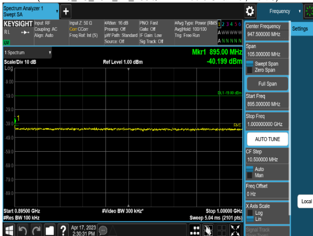
Plot 8-626. Conducted Spurious Emission Plot 895 MHz to 1 GHz (LTE B5_1C_10M_4T_256QAM - Middle Channel, Port 0)
