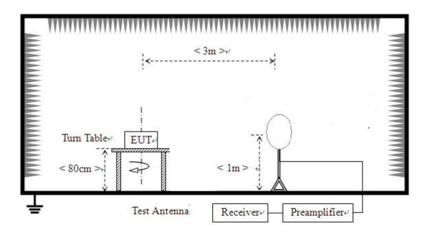
For radiated emissions from 30MHz to 1GHz
