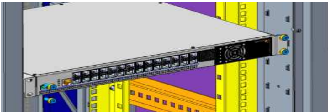
Figure 37. Rack Installation - Step 2
