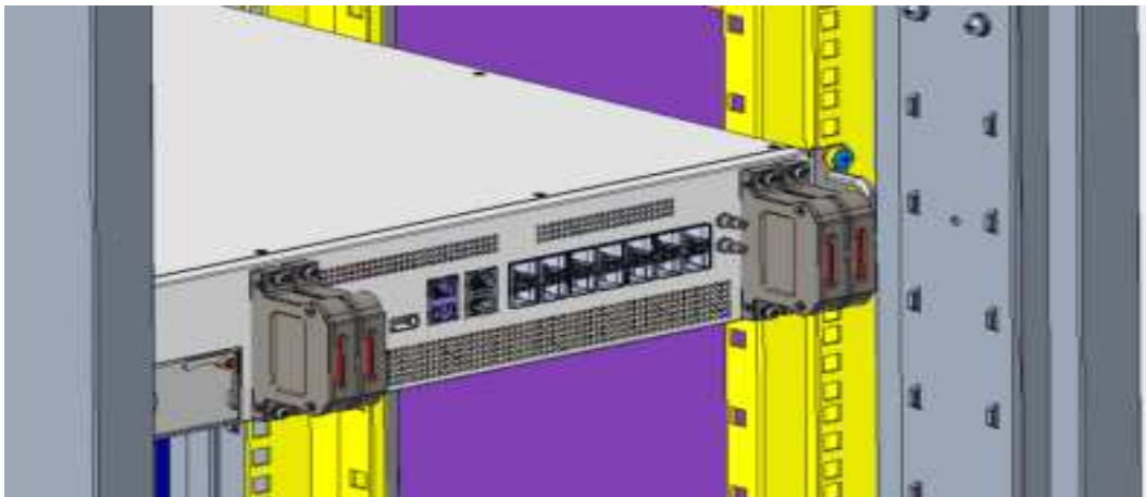
Figure 34. DCU RF Cable Plug Installation
