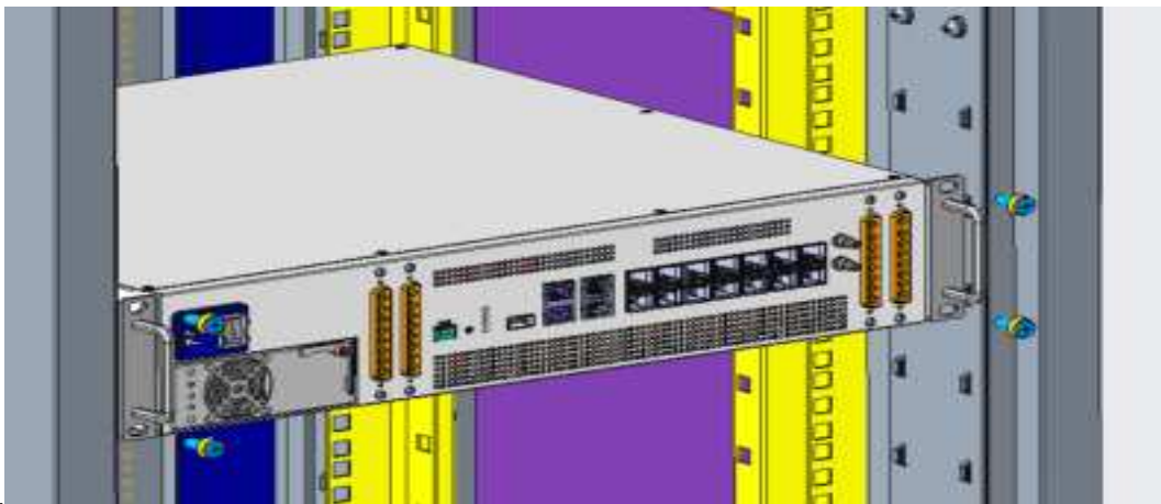
Figure 33. Installation Diagram of DCU in the Rack
