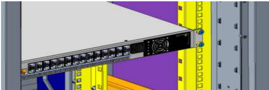
Figure 38. Rack Installation - Step 3
